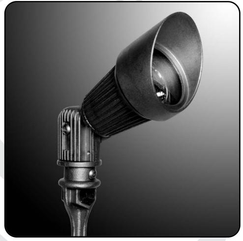
Guarantee quality and function when you specify the solid brass Okeeffeliter. Backed by a lifetime warranty, this specification-grade fixture is ideally suited for the commercial environment or high-end residential project. The ribbed construction allows for heat dissipation of all MR-16 lamps, and maximizes rated lamp life and constant color rendition.
